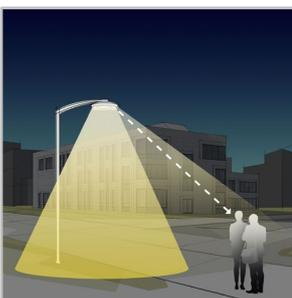
Because of the lower installation height compared to road lighting, visual comfort is an essential aspect of urban lighting. Schröder designs lenses and accessories to minimise any type of glare (distracting, discomforting, disabling glare and blinding glare). Our design offices harness a range of possibilities to find the best solutions for each project and ensure that we provide a gentle light that delivers the best night-time experience.
