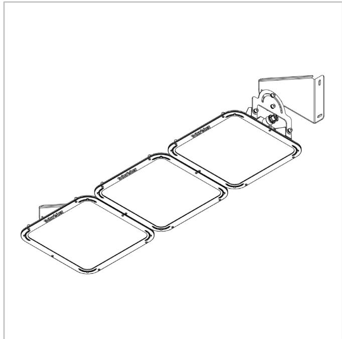
TFLEX MODULE | Hook fixation - more details in the installation sheet
